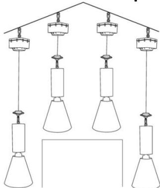
When lowering, the lift stops automatically if the decent is interrupted or when it reaches the ground.
