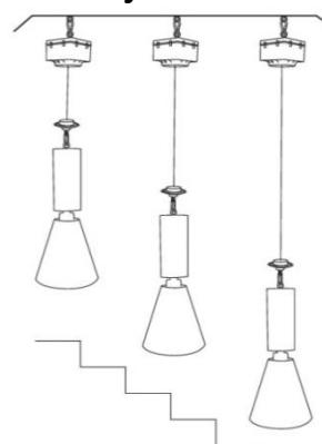
Each lift can be set to stop at the users desired lowering height. This can be stored in the lift for future operations
