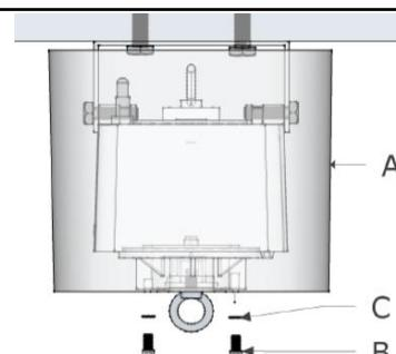
**AH C** : Used to cover surface mounted lifts, can also be painted to match ceiling colour.
