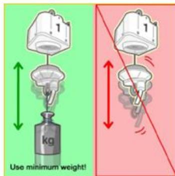
DO NOT operate the lift without the minimum weight or the lift will fail!
