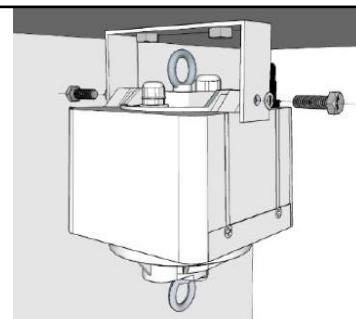
**MB C** : Used to securely mount the lift to the ceiling substrate with two points of fixing.
