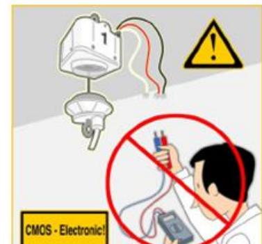
DO NOT apply any external voltage to the signal control wires!
